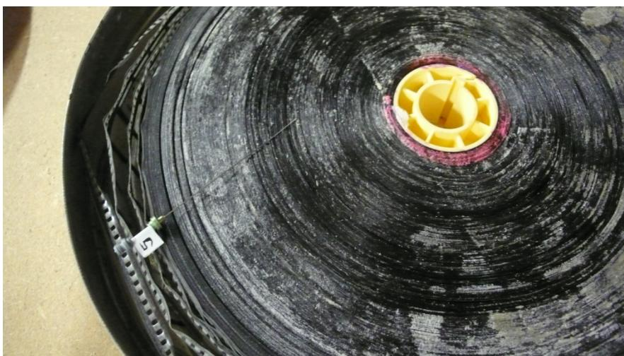
Detail: A highly degraded roll of 35mm cinematographic film, suffering from vinegar syndrome and plasticiser exudation
