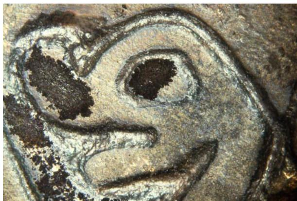
Figure 7: ‘Black spots’ covering large parts of a medieval bronze fibula (KN 116)<sup>8</sup>
